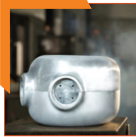
245Kv Core Housing
